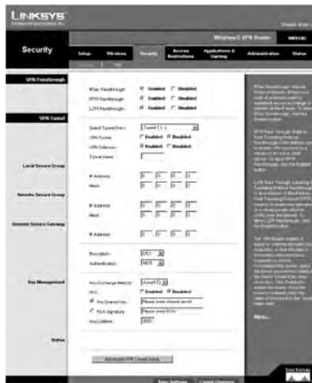
Figure 21.43: The WRT54G VPN settings
