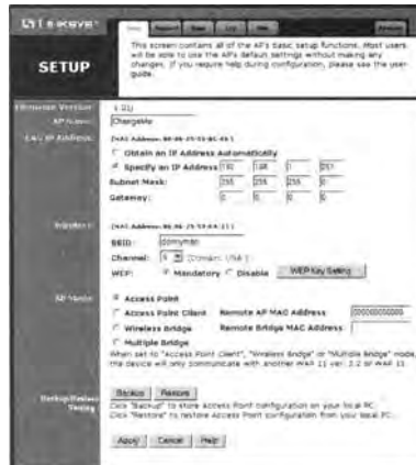
Figure 20.5: Making WEP mandatory on the Linksys WAP11
