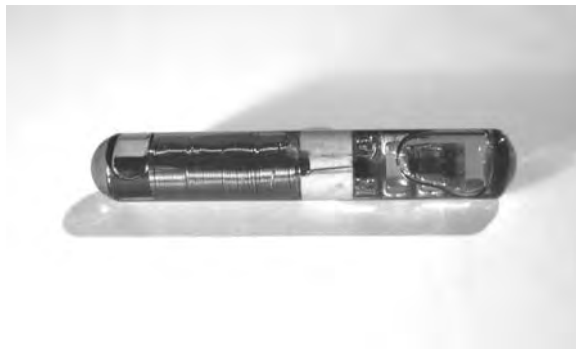
Figure 24.8: A passive tag's internal components
