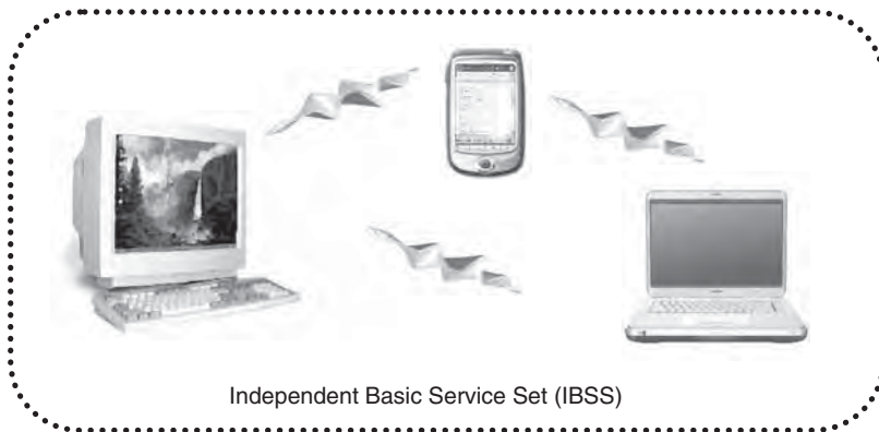
Figure 6.2: Ad-hoc mode topology
