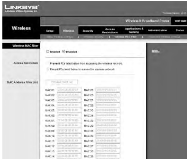
Figure 22.3: Adding MAC addresses to your wireless router
