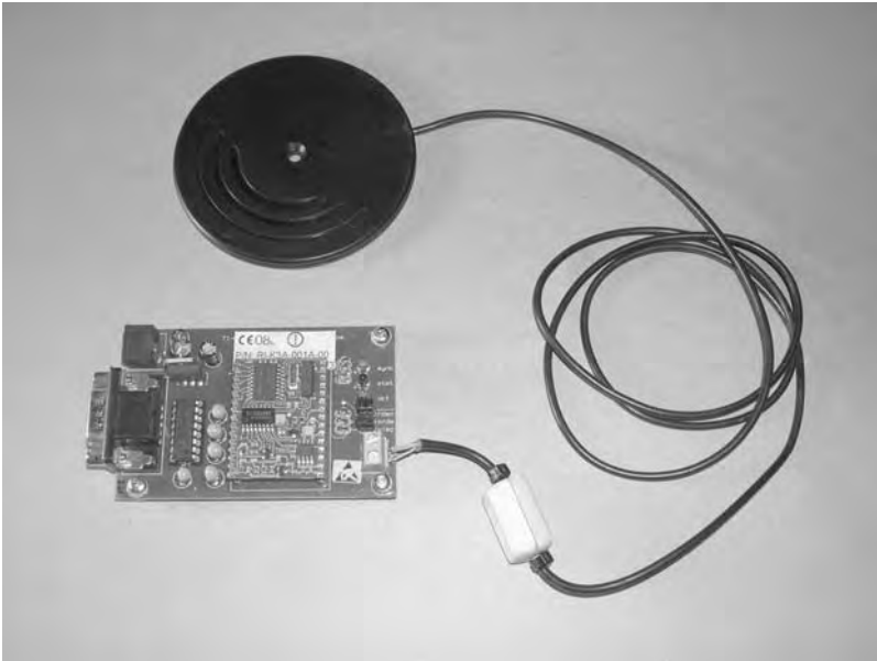
Figure 24.2: RFID reader including the antenna and electronics package
