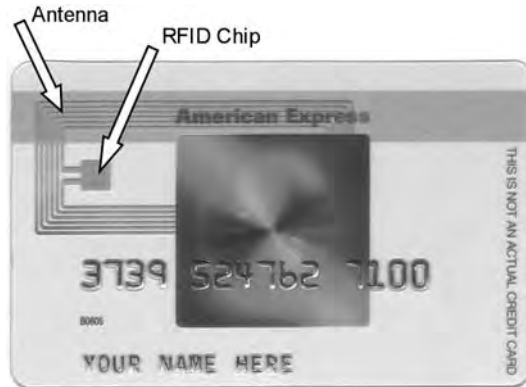
Figure 24.7: Fake credit card showing the RFID chip and antenna
